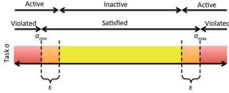
Fig. 1: Definition of main regions in set-based control for a task with an upper and lower bound. The task is considered active when it is within an interval \varepsilon from the limits.
