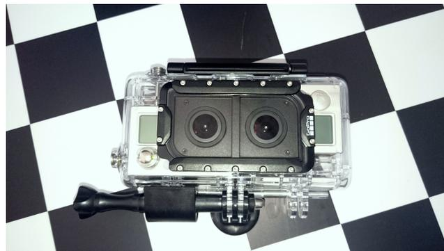
Figure 20: The stereo system consisting of two Gopro Hero3+ Black Edition cameras in a Gopro Dual HERO underwater housing.
