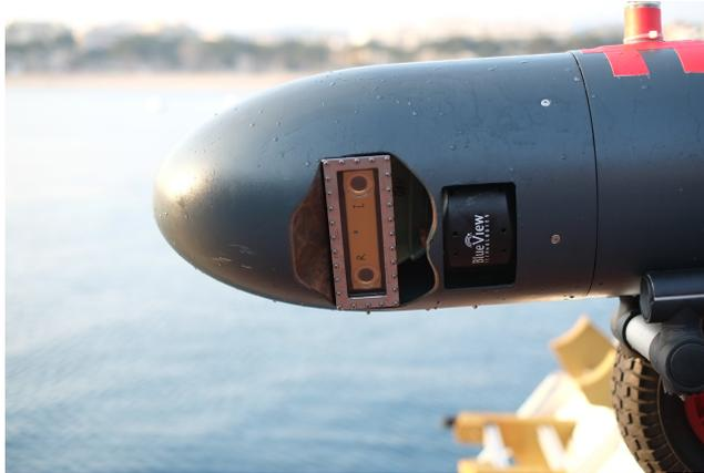
Figure 16: A Point Grey Bumblebee 2 stereo camera and Blueview MB2250 Multibeam Echosounder integrated on a Seacat from ATLAS Elektronik.
