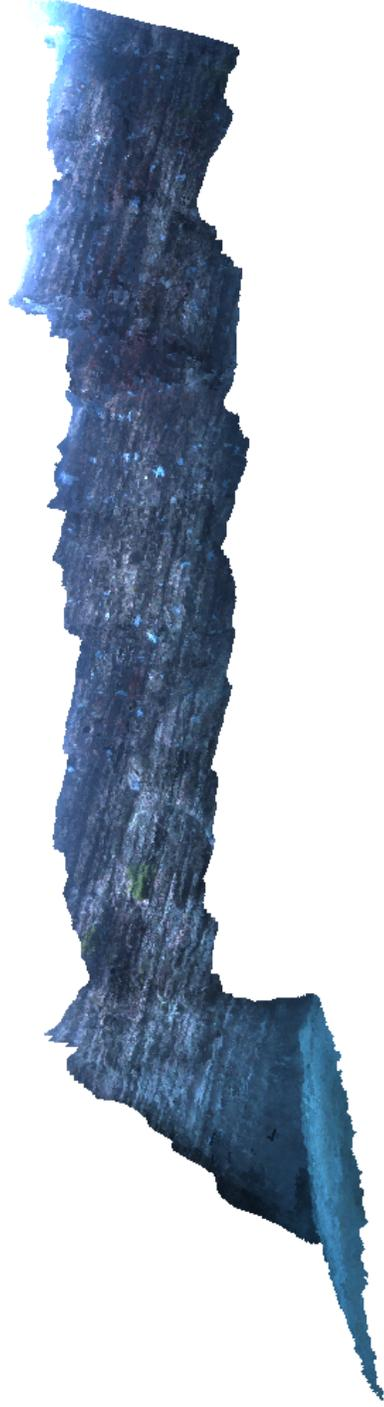
Figure 15: A 3D map generated from 350 stereo based point clouds from a Bumblebee camera on a Sparus vehicle of the University of Girona. The consistently dense stereo data in all stereo computations indicates high rectification accuracy.
