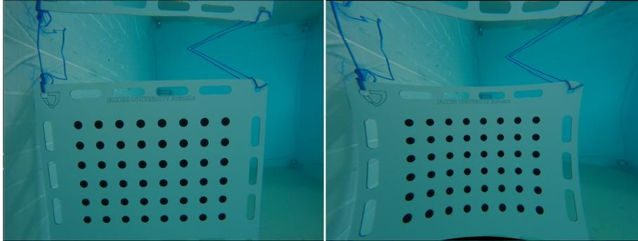
Figure 22: For the GoPro data, the in-air calibration leads to such severe distortions that the stereo processing is completely failing in this case. On the left, an example GoPro image from a test sequence is shown; on the right, the “corrected” image based on in-air calibration is shown.
